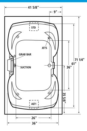
Note: Rough-in measurements may vary + - 1/4". Pump locations are shown for clarity. STD-standard pump location. ALT1- optional alternate pump location. If a factory installed nailing flange is added to a unit, add 1/8" to each side flanged.
