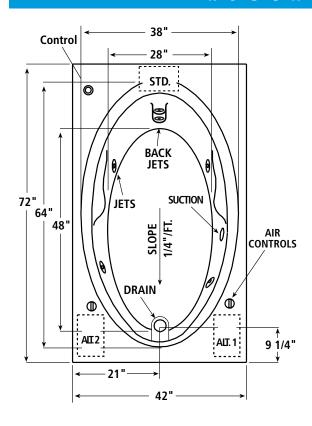
Note: Rough-in measurements may vary + - 1/4". Pump locations are shown for clarity. STD-standard pump location. ALT1 and ALT2 - optional alternate pump locations. If a factory installed nailing flange is added to a unit, add 1/8" to each side flanged.
