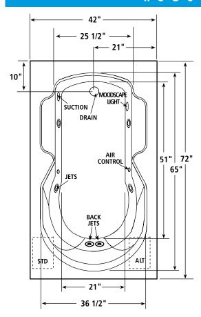
Note: Rough-in measurements may vary + - 1/4". Pump locations are shown for clarity. STD-standard pump location. ALToptional alternate pump location. \*\* Electronic SimpleSelect located on (Std or Alt) corner of deck. If a factory installed nailing flange is added to a unit, add 1/8" to each side flanged.
