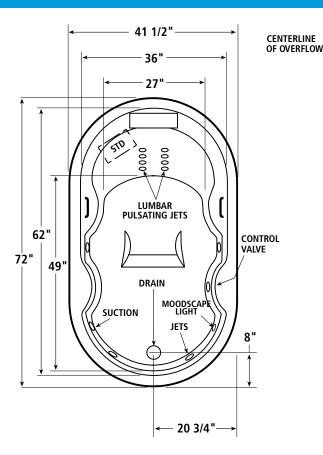
**INSTALLER NOTE:** Due to the freeform shape of the tub shell, it is recommended that the tub be on the job before making the final cut-out for drop-in installation.
