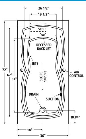
Note: Rough-in measurements may vary + - 1/4". If a factory installed nailing flange is added to a unit, add 1/8" to each side flanged.
