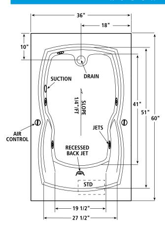
Note: Rough-in measurements may vary + - 1/4". If a factory installed nailing flange is added to a unit, add 1/8" to each side flanged.
