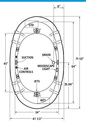
Note: Rough-in measurements may vary + - 1/4". They may vary 1/4" (+/-). Pump locations are shown for clarity. STD-standard pump location.ALT1-alternate pump location.
