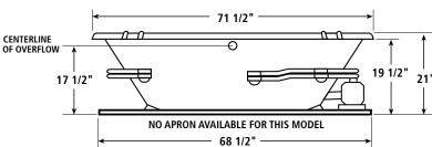
INSTALLER NOTE: Due to the freeform shape of the tub shell, it is recommended that the tub be on the job before making the final cut-out for drop-in installation.
