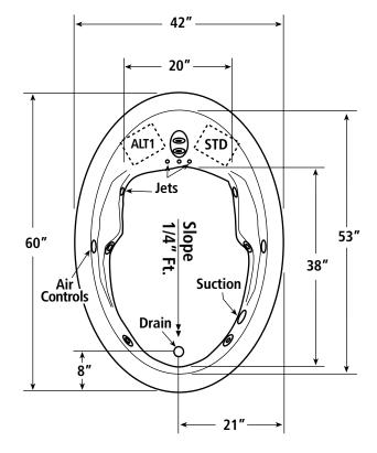
Note: Rough-in measurements may vary + - 1/4". Optional pump locations. Shown for clarity. STD-standard pump location. ALT1-alternate pump location. Specify one location when ordering. Nailing flange not available on this unit.
