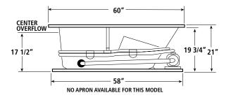
**INSTALLER NOTE:** Due to the freeform shape of the tub shell, it is recommended that the tub be on the job before making the final cut-out for drop-in installation.
