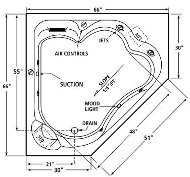
Note: Rough-in measurements may vary + - 1/4". Pump locations are shown for clarity. STD-standard pump location. ALT1- optional alternate pump location. If a factory installed nailing flange is added to a unit, add 1/8" to each side flanged.
