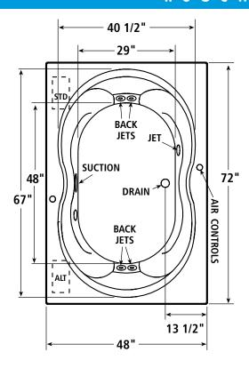
NOTE: Rough-in measurements may vary 1/4" (+/-). Pump locations are shown for clarity. STD-standard pump location. ALT-alternate pump location. \*\* Electronic SimpleSelect Control located on (Std or Alt) corner of deck.
